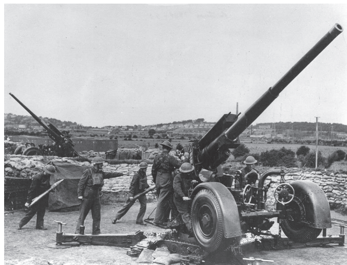
DEFENCE: A British 3.7in AA gun, the equivalent of the German 88mm
